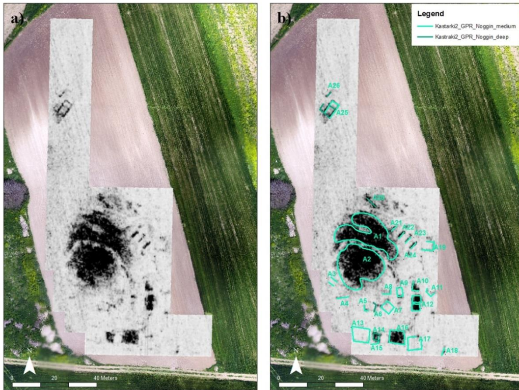
Figure 10: GPR results interpretation where (a) is the georeferenced slice at 120-130cm superimposed on the UAV image, while in (b) the outlines of the identified anomalies.
